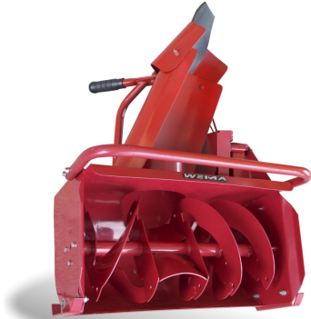
Name: Snow Blower Matching model: WMX720 WMX610 Working width: 60~70cm Working speed: 1200RPMs
