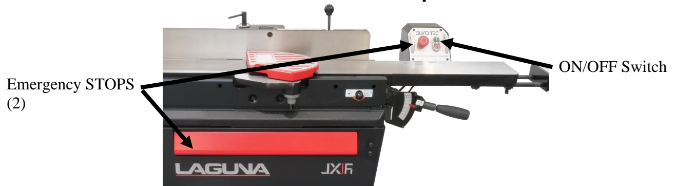
Figure 7: Control Panel & E-STOPS
