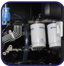
Fuel particle separator filter
