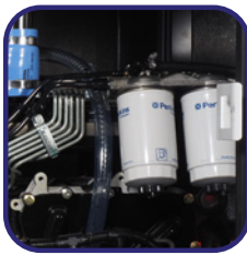
Fuel particle separator filter
