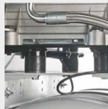
Engine/unit base installed on 4 anti-vibration rubber dampers for less vibrations, reduced noise and longer service life (only on Diesel models)
