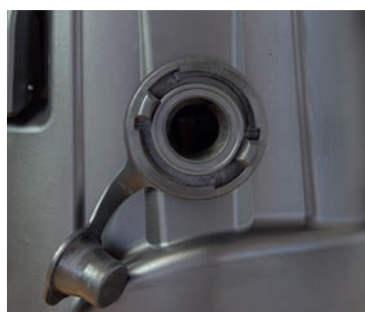
C-pipe connection for wastewater
